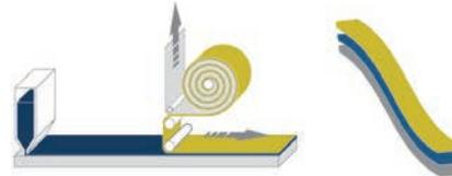
Extrusion lamination with PVC
